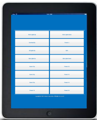
Event staff at the War Memorial use an iPad with 16 present buttons for direct control.
