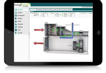
Autani's wireless sensors and ductwork probes can measure temperature, humidity, differential pressures to maintain comfort in the store's sales environment, and that the HVAC equipment is optimally performing as designed with:
